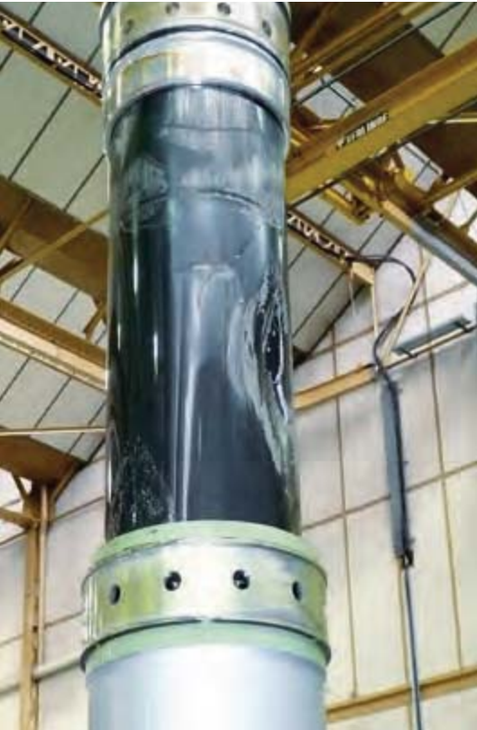
Figure 3 Damage on the aircraft following the hard landing: aircraft's Landing Gear
