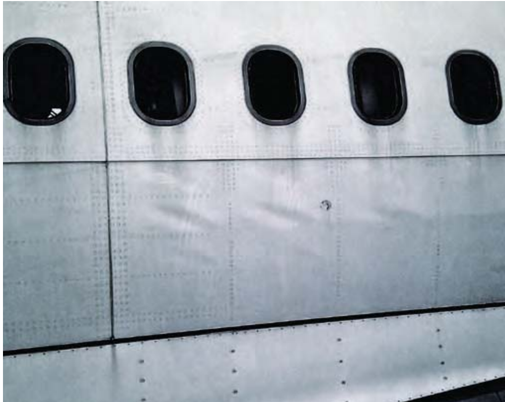
Figure 4 Damage on the aircraft following the hard landing: ripples on the fuselage
